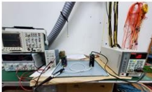
PSE output power measurement using short cable ( left ) and long cable ( right ).
