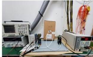
PSE output power measurement using short cable ( left ) and long cable ( right ).
