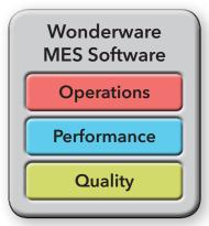
**Quality operations** integrated with production work order execution for quality test and sample specification management and execution of quality sampling procedures for quality data collection, either direct from process equipment or through operators with sample plan procedure enforcement.
