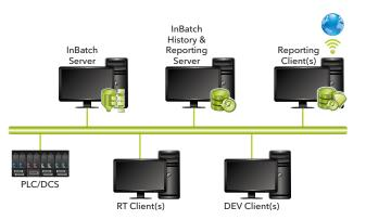
InBatch software's batch management system consists of scheduling, initializing, equipment arbitration, allocation and release, coordinating the processing of batches with the control system, interfacing with operator runtime clients, and directing batch activity, material consumption and production records to the historical database.
