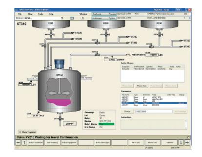
**InBatch optimizes throughput and equipment utilization.** InBatch's uniqueness is in its comprehensive process capabilities model, going beyond ISA-88 to include connections and transfers. This enables the batch engine to manage flexible product paths, allowing simultaneous multi-product and multi-stream batch execution on shared equipment and connections.
